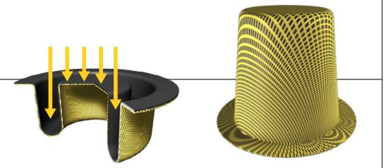
In the axial direction, fabric provides high resistance to elongation and furnishes the tensile strength that enables the seal to withstand high differential pressures.
